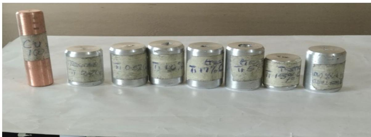
**Figure 2:** Developed beta phase Titanium copper specimens and copper specimen
