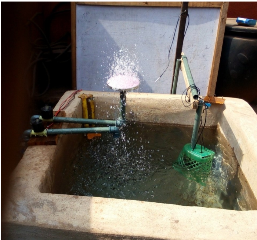
Figure 3: Snapshot of the Process of Replenishing Discharged Pond Bottom Water by the System
