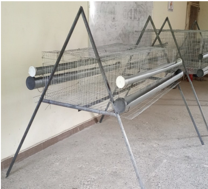
Figure 14: Side view of two-way battery cage for layers showing the feeding, drinking and automated egg collection unit
