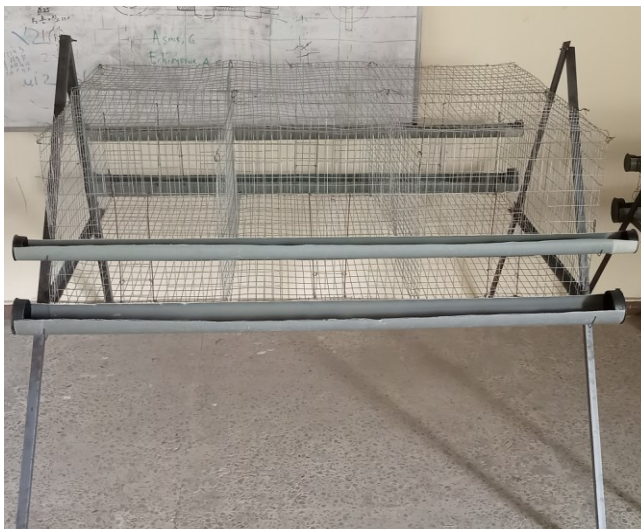
Figure 12: Front view of designed and built two (2) ways battery cage with three compartments (tiers) for general birds
