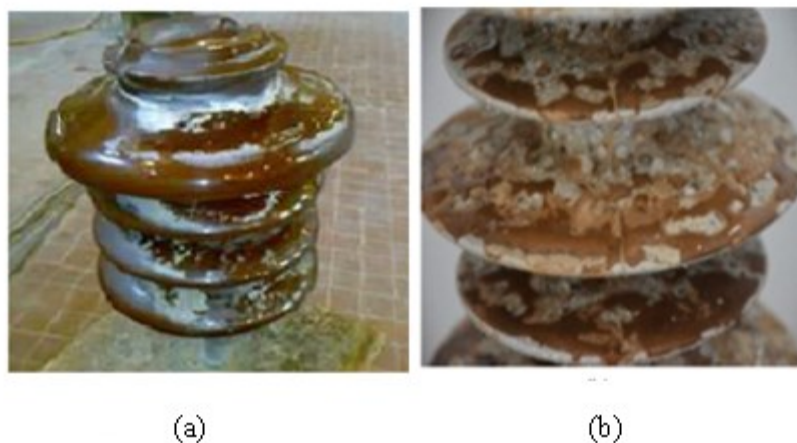
Fig 2: (a) Pollution Degraded Insulator (Hossam-Eldin, et al. , 2011) (b) Insulators given fly ash pollutant (Negara, et al. , 2021).
